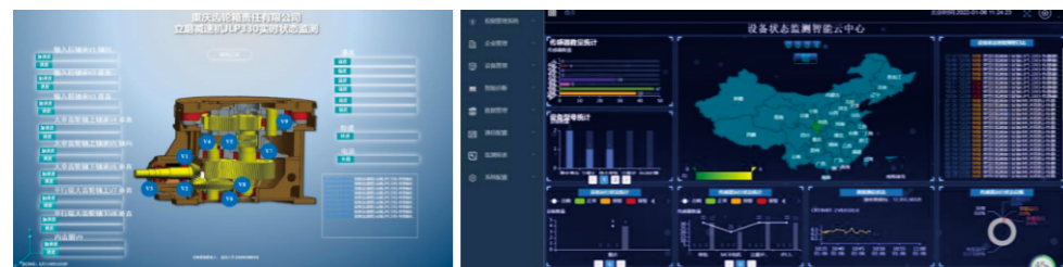
立磨减速机状态实时状态监测 Real-time monitoring of state of vertical mill reducer
